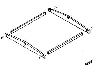
1. Slot joists into gable ends, bevelled side uppermost. Nail in position, using 1" nails.
