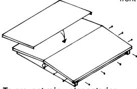
To prevent rain water entering the roof by capillary action it is a good idea to seal roof boards and ridge bar on to the roof using a silicone sealant.
