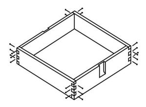
1. Glue and nail together the four side walls with the vents opposite each other facing out, using 1.5" nails.
