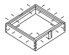
3. Check roof is square. Using drawing pins, pin the ventilator mesh over slots in top board.
