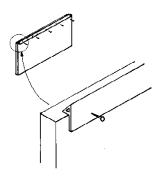
1. Bradawl the runners to prevent splitting. Nail the runners centrally on one side of the inside walls. using brass escutcheon pins.
