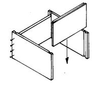
Push inner boards into groove, ensuring top of runner coincides with mark. (Shown below)
