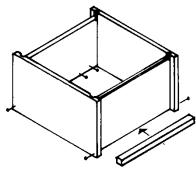
6. Nail top lath from the inside, with spacer slot uppermost, flush with the top of the inner wall, using 1" Nails. Ensure nails miss the spacer slot. Nail end laths in position flush with top edge of box, using 1" nails
