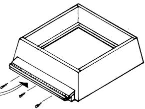
Place lift flat on bench and position porch centrally to one of the sides, ensuring base of porch is flat on bench. Screw porch in place, using 1.5" black japanned screws.
