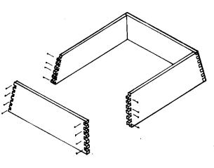
1. Push the four walls together. Nail corners using 1.5" nails. NOTE: the top and bottom edges of lift are bevelled thus ensuring that, as the lift slopes inwards, the top and bottom are horizontal.
