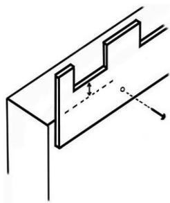
N.B. If assembling a Budget super, there are no saw cuts in the inner wall and frame runners are not used. In this case the castellated spacers are nailed centrally on one side of the inner walls, using brass escutcheon pins. The castellated spacer cut-outs must project above the inner wall by 1/4".
