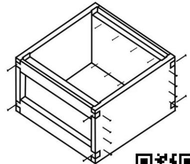
5. Nail through outer walls into inner walls using 2" nails. Nail locking bars from inside  $3/16"$  down from runner, using  $1\ 1/2"$  nails.
