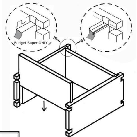
3. Apply glue to the grooves in the outer walls and then push the inner boards into the groove, ensuring top of runner coincides with mark. If assembling a Budget super, the top of castellated spacers must be flush with the top of box.
