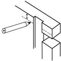
2. Mark the outer wall  $7/16"$  down, adjacent to the long groove
