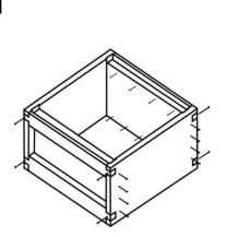
5. Nail through outer walls into inner walls using 2" nails. Nail locking bars into position using 2" nails. Nail locking bars from inside  $3/_{16}$ " down from runner, using 1  $1/_2$ " nails.
