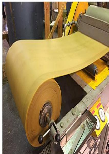
Our wax is now liquefied in powerful electric vats, 1500kgs at a time. Most of the time we clean the wax by simply floating it on water. By this simple and effective method of sedimentation it is possible to clear the wax of all solid debris. Nothing is added to our wax to
