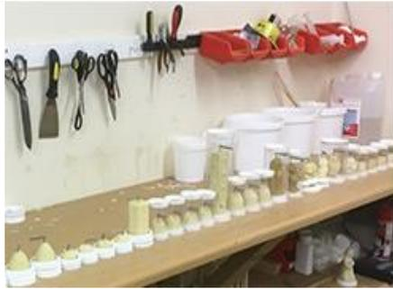
The mould masters are then setup ready to pour the silicone. We use a very high-grade silicone which has been proven over the years to give best results with the moulds lasting many years.
